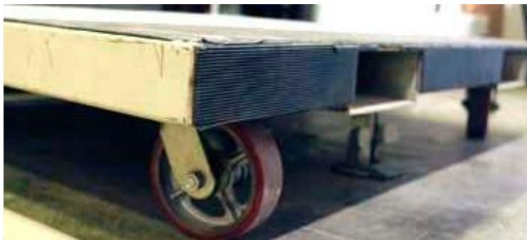
Platform side view, with casters, brake & forklift slots
