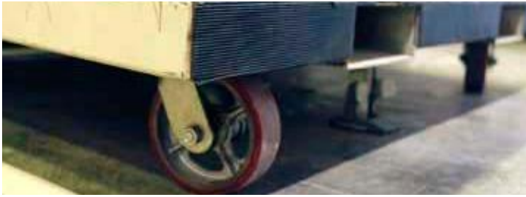
Platform side view, with casters, brake & forklift slots
